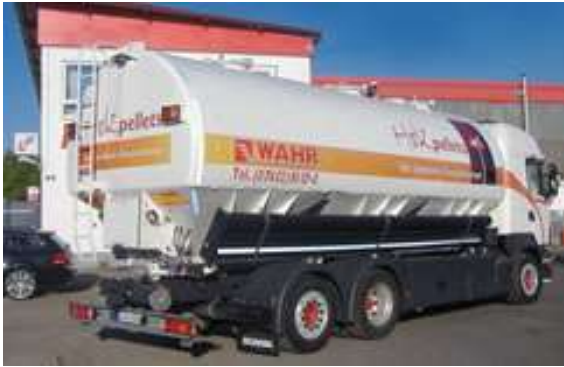
Figure 18: Truck for loose pellet delivery
