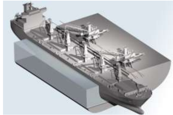
Figure 14: Pneumatic ship pellets unloading system (www.bulkinside.com)
