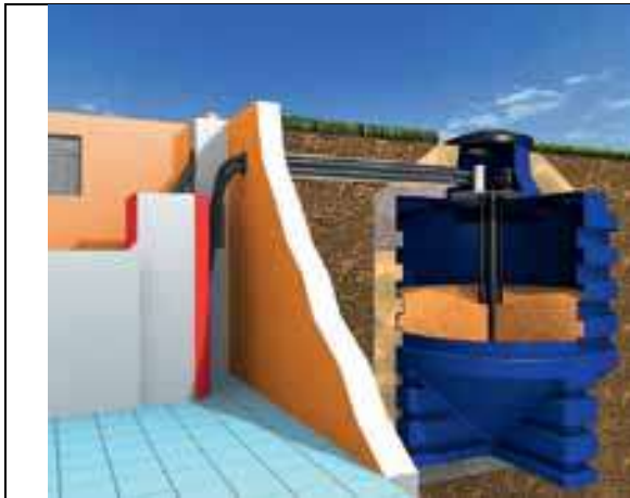
Figure 9: Below-ground silo made of synthetic materials, discharged from the bottom of the storage (DEPV 2011)
