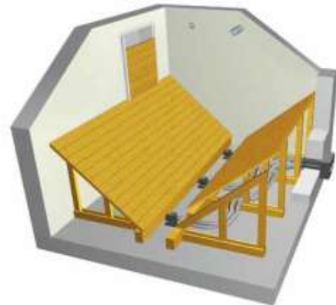
Pellet silo with inclined bottom and suction extraction
