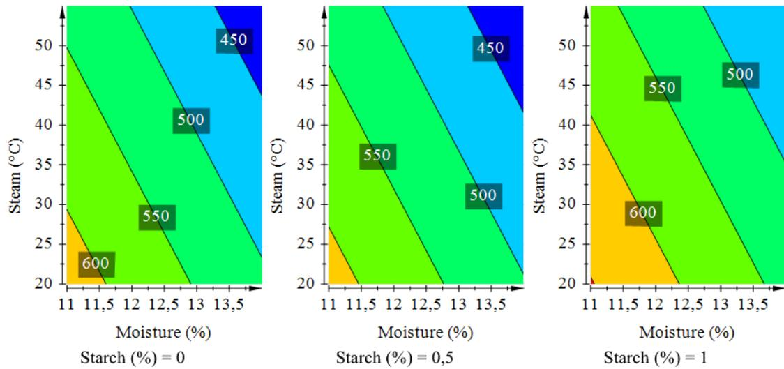
**Figure 4.** Prediction plot for bulk density ( $\text{kg/m}^3$ ) when starch is used.
